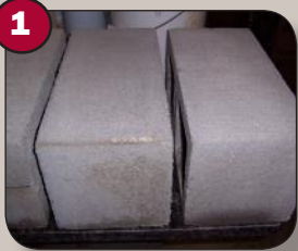
Test samples of silicate left on concrete.
